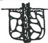
BIG POSTS FOR TARPS AND POSTS FOR OFF-THE-GROUND STRUCTURES LIKE SHELVES, TABLES, RACKS NEED TO BE STABLE. IT'S BEST TO DIG A BIG HOLE, PUT THE POLE INTO THE CENTRE AND THEN SUPPORT IT WITH ROCKS AND SOIL WHICH GET POUNDED IN.
